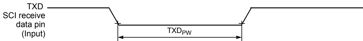
Figure 10-17 TXD Pulse Width
